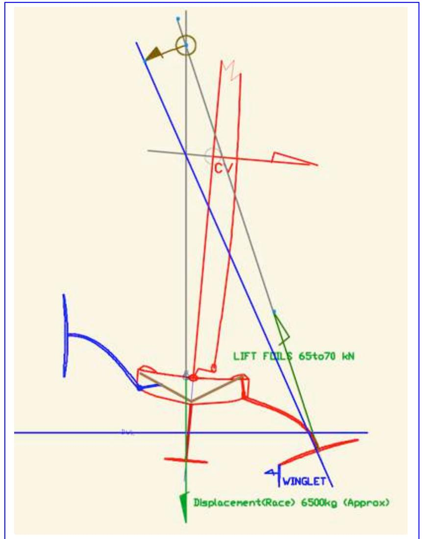
The solution will probably involve installing a Winglet at the end of the foil.
