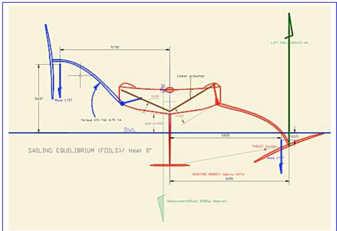
Contrary to what is said, the raised foil, which is windward, does not increase stability because there is one foil on each side (BB and TB). The resultant of the masses of these two foils is even downwind, because the lever arm of the active foil is more important than that of the raised arm!!
